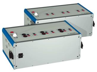
Controlling the source is carried out in a similar way as to control the reference meter, by use of one of the PRS 600.3 touch displays or via RS 232 C.
